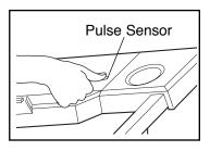
will be restricted, and your pulse will not be detected. Next, raise your thumb slightly until the heart-shaped indicator in the pulse display flashes steadily. Hold your thumb at this level. After a few
